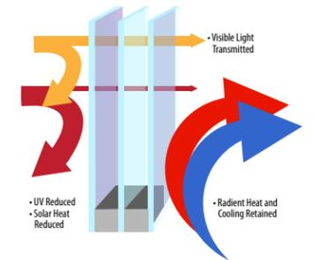
In climates where heating and cooling are the primary concern, HeatSeal® Glass products are designed to take advantage of free solar heat, resulting in higher inside glass temperature. Passive solar and thermal insulation reduce the draft sensation caused by cold glass surfaces, providing windows that reduce heating costs.
