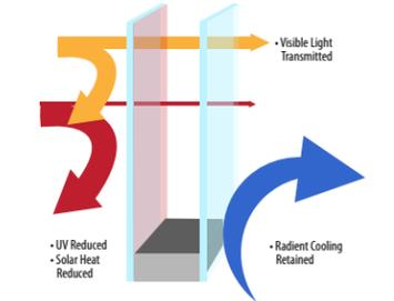
In climates where cooling is your main concern, SunSeal® Glass products are designed to reduce solar heat while still providing color-neutrality. This solar control property, combined with thermal insulating benefits, results in beautiful, natural-looking glass that helps keep air conditioning costs low.
