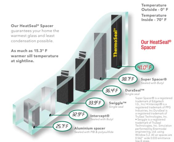
Examples of Condensation: A good quality spacer can significantly reduce condensation in comfortable humidity levels. Water and ice forming can lead to mold growth.
