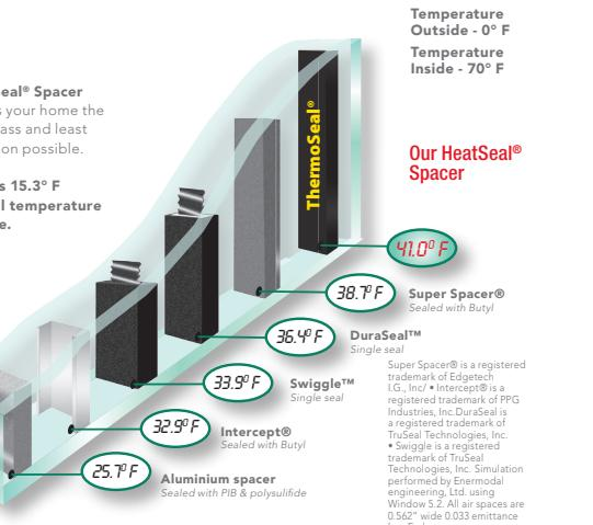
Examples of Condensation: A good quality spacer can significantly reduce condensation in comfortable humidity levels. Water and ice forming can lead to mold growth.
