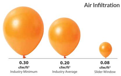
The results are based on a tested window sample by AAMA testing window guidelines. Title of Test & Method: Air Infiltration - ASTM E 283 75 PA - (1.6 psf) 25 mph
